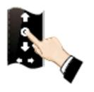
Start the motor, press "STOP" on the program controller for 5 seconds. The motor is in programming mode for 30 seconds.
